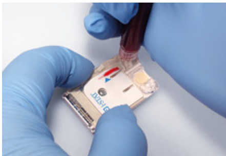
Step 1: Scan cassette bar code, insert 2-3 drops into cartridge
