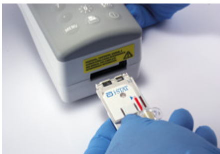
Step 2: Close cartridge and insert into the i-STAT handheld
